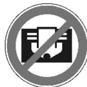
The **built-in thermal protection switch disconnects the ERS Heatscreen from the mains at a temperature of approx. 140°C**, after a cooling phase (approx. 10-15 minutes) to approx. 90°C it switches itself back on again. **It is essential that you eliminate the cause of the overheating** (cover up, block) so that the ERS Heatscreen can work normally again and there is no reduction in service life due to the high thermal load and the switching of the thermal protection switch.
